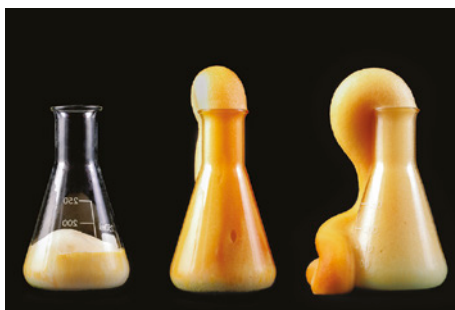
FIGURE 5.3.1 The 'elephant's toothpaste' demonstration involves a redox reaction in which hydrogen peroxide is both the reducing agent and the oxidising agent.
