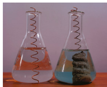
FIGURE 5.1.11 When a strip of copper wire is suspended in a solution of silver nitrate in the flask on the left, long crystals of silver metal start to form. In the flask on the right, the copper has displaced the silver from the solution.
