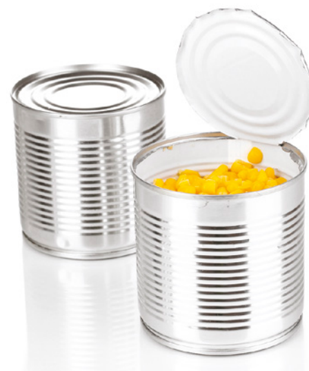
FIGURE 5.1.18 These food cans are made from steel that has been plated with tin to prevent them from corroding.
