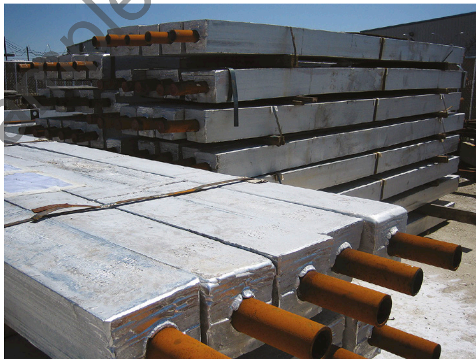
FIGURE 5.1.21 These aluminium sacrificial anodes are attached to the underwater steel structures of offshore gas platforms to protect them against corrosion.
